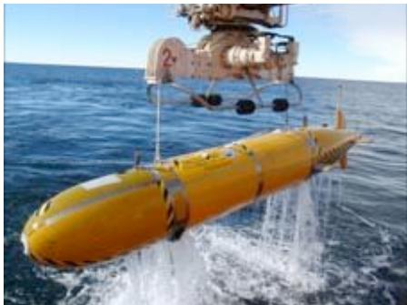
The AUV has the capability to dive to depths of 1,600m below the surface
