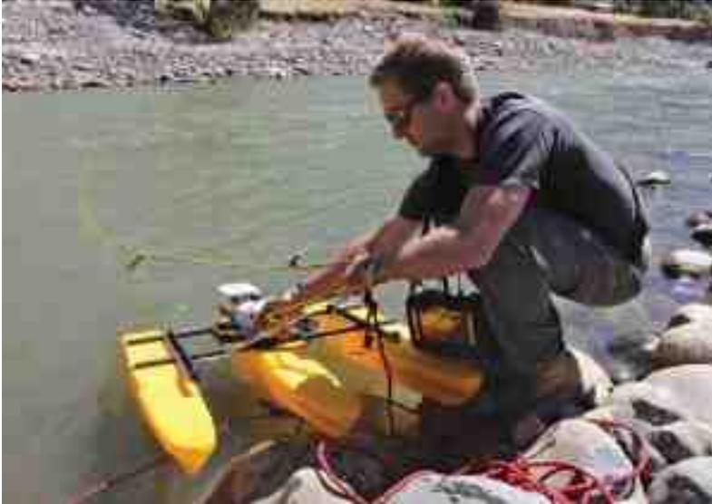
A researcher launches a doppler device to measure stream discharge.
