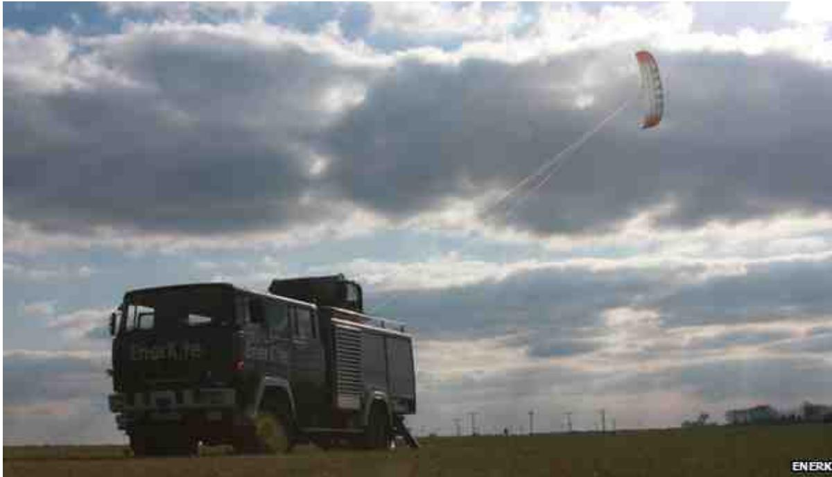
EnerKite generates electricity by using the wind to reel out a specially designed carbon-fibre wing
