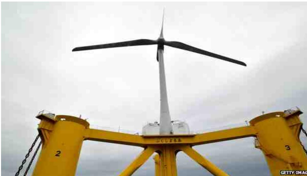
Floating turbines offer great potential for wind power where sea beds drop away very quickly. Not only, then, do floating turbines open up possibilities for wind generation in new places, but they hold some advantages over their fixed counterparts. They can be built and assembled onshore and then towed out to sea, and if repairs are needed they can simply be towed back again, making maintenance easier and cheaper.
