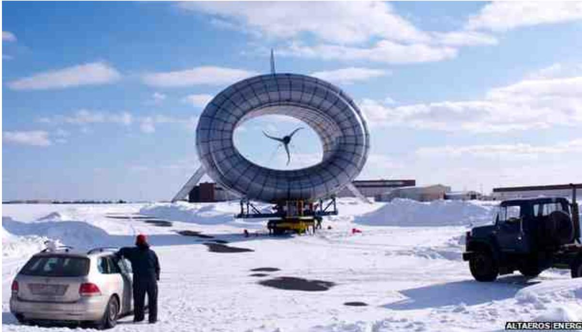
Altaeros Energies' BAT uses helium gas to take the turbine hundreds of metres into the sky. The notoriously secretive Google X is also getting in on the act, having bought wind power company Makani in 2013. Its solution involves a tethered, carbon fibre glider flying in circles at an altitude of up to 350m, carrying up to 8 small turbines producing 600KW of power. Makani claims each glider can generate 50% more energy than a traditional, fixed turbine.
