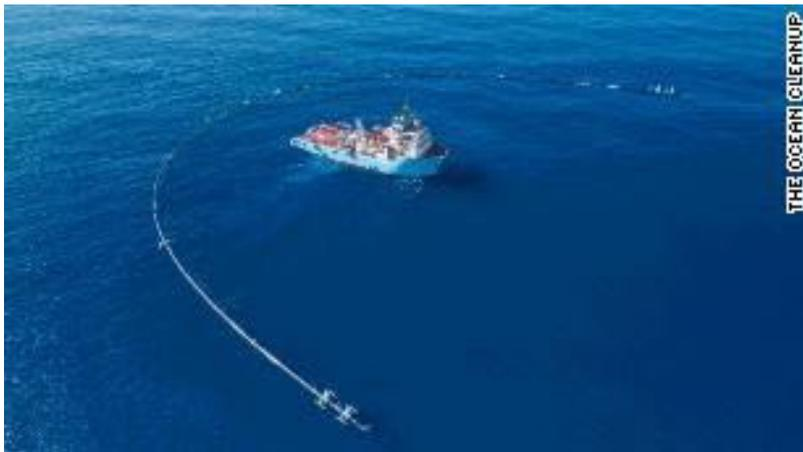
The Ocean Cleanup uses a U-shaped pipe to collect plastic. The company's goal is to clean the world's oceans.
