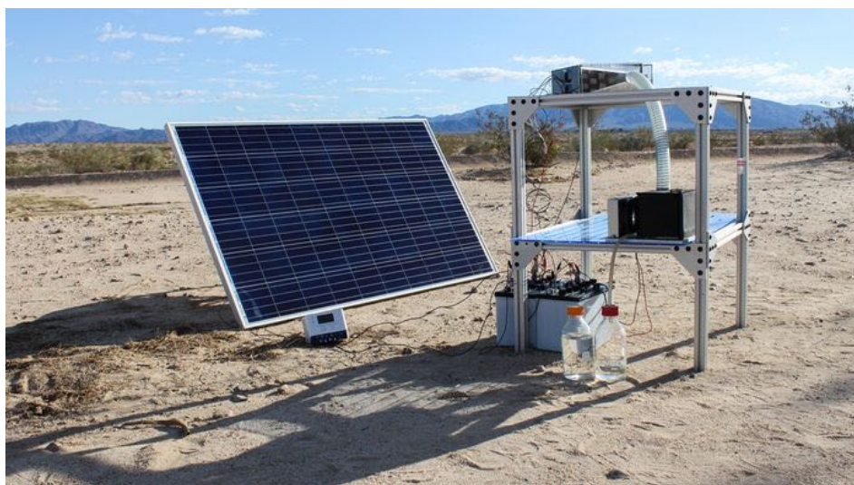
A solar panel powers a device that harvests water from the air in California's Mojave Desert. MATHIEU PRÉVOT
