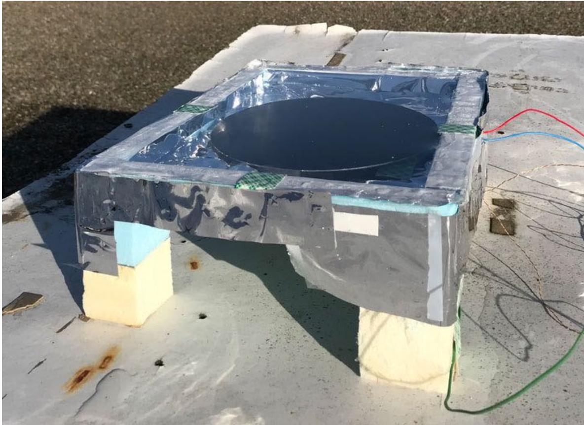
A device that uses the night sky to generate electricity (pictured) powered a small LED bulb in one rooftop experiment.
