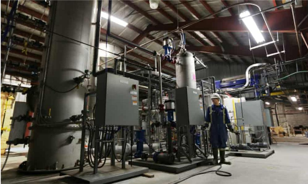
The Canadian firm Carbon Engineering's pilot plant pellet reactor and associated equipment. Photograph: Carbon Engineering
