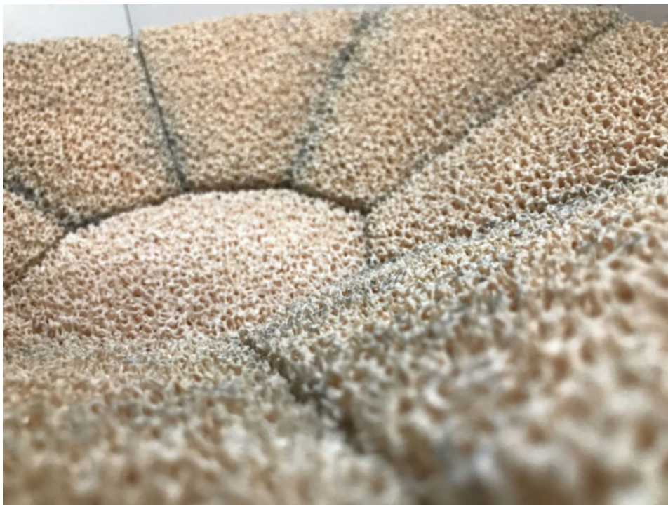
Within the solar reactor, porous ceria (shown) gets heated by sunlight and reacts with carbon dioxide and water vapor to produce syngas, a mixture of hydrogen gas and carbon monoxide.
