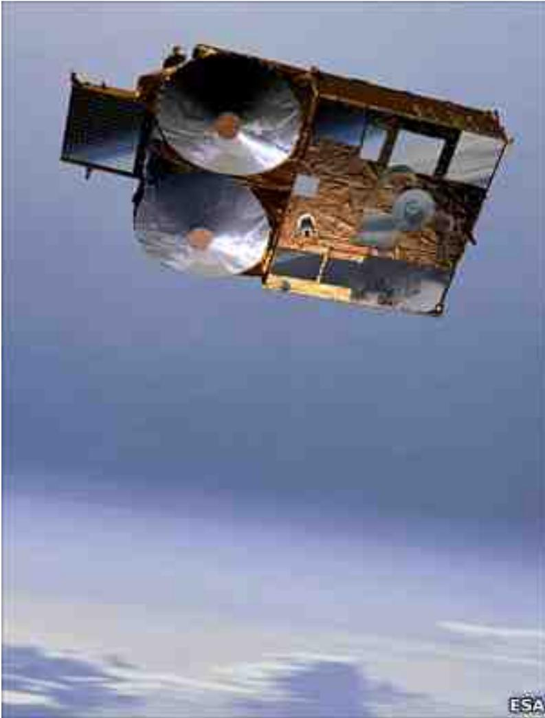
Cryosat's double antenna
