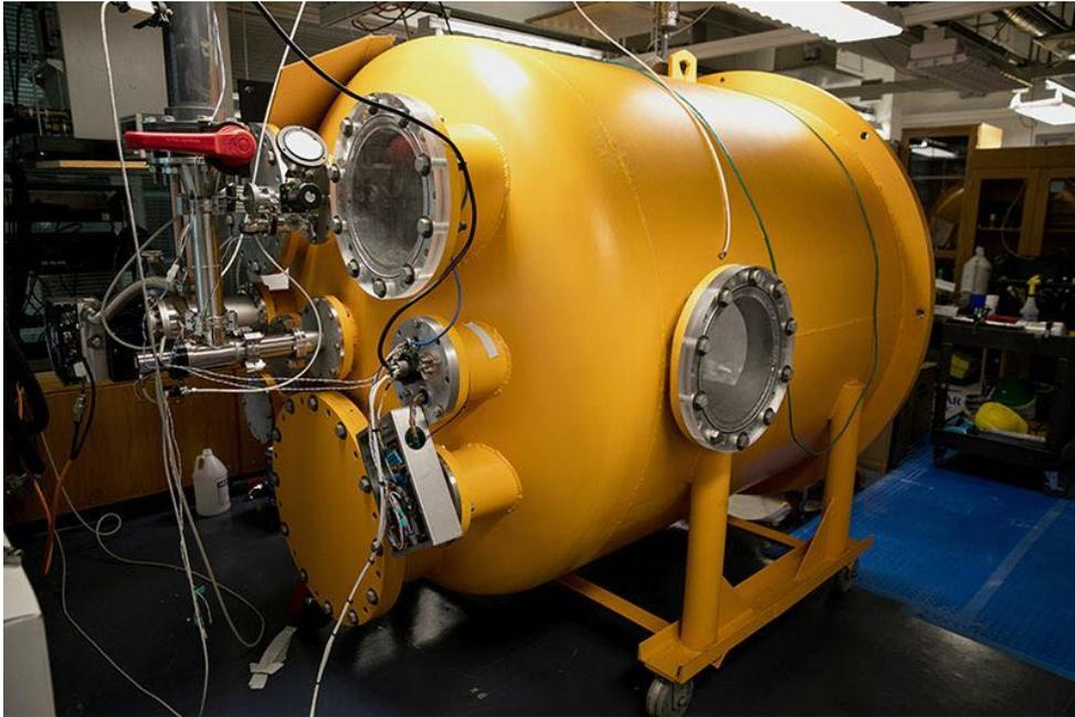
An environmental chamber to test instruments used in the SCoPEX field mission. Credit: Kayana Szymczak for *Nature*
