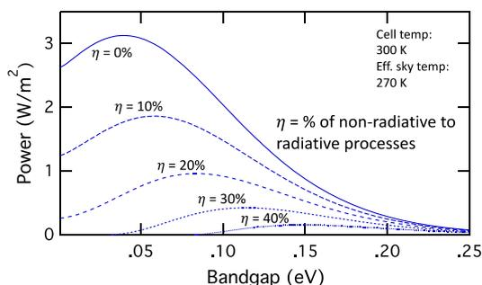
**Figure 6.** Power output for different percentages of nonradiative generation,  $\eta$ , for a thermoradiative device operating at 300 K exposed to a sky with effective temperature of 270 K, simulating clear sky conditions.<sup>22,23</sup>
