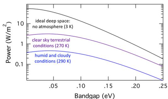
**Figure 2.** Maximum power density vs bandgap energy for a 300 K terrestrial cell and three selected sky conditions, modeled with effective sky temperatures. The ideal case is a cell directly accessing the darkness of space at 3 K, 270 K simulates clear terrestrial conditions, extrapolated from maximum radiative cooling estimates,<sup>22,23</sup> and 290 K corresponds to humid and overcast conditions.
