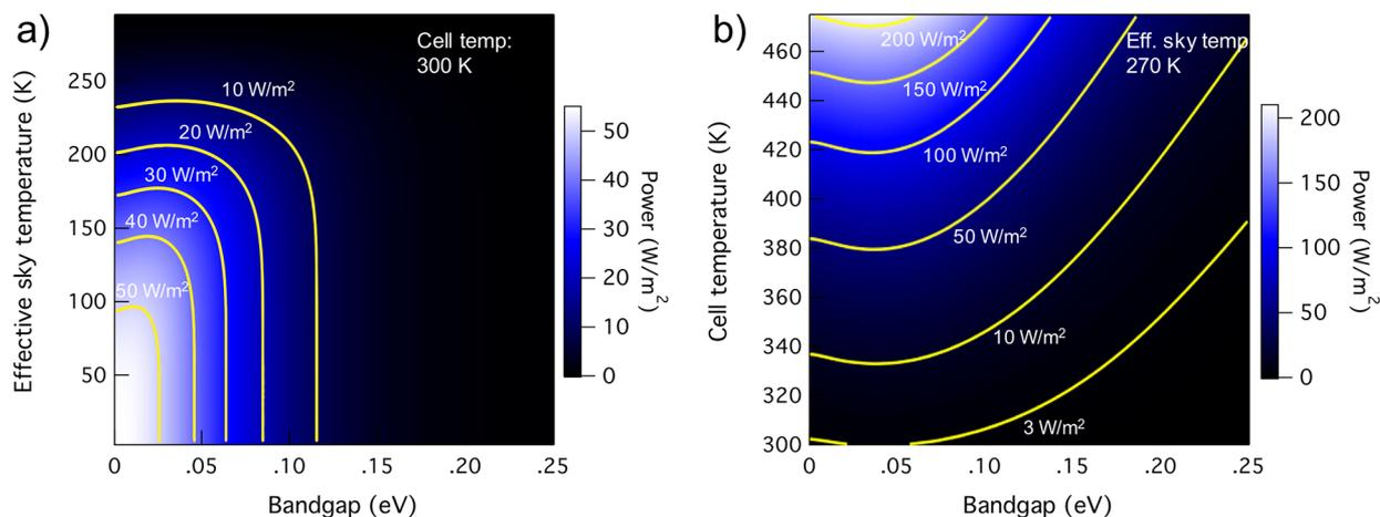
**Figure 5.** (a) Maximum power output of a thermoradiative cell, held at 300 K, whose semiconductor bandgap ranges from 0 to 0.25 eV for effective sky temperatures 3 to 295 K. The optimal bandgap increases as effective sky temperature increases, showing broadening contour lines. (b) Maximum power output of a thermoradiative cell at a range of temperatures, coupled with the sky at an effective temperature of 270 K, simulating clear sky conditions.<sup>22,23</sup>
